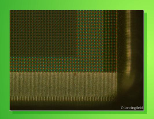
A CMOS sensor under a microscope looks like many red green & blue dots
